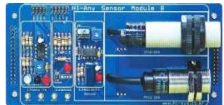
▶ PAMS-AnyLab V1.0-8 (근접 / 용량 Sensor 4종) (Photo TR, Magnetic HW200A, Proximity Capacitive, Cylindrical)
