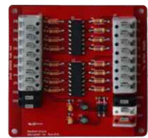
▶ PAMS-AEB V9.3-8 (Photo Coupler Control Board)
