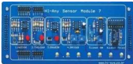
▶ PAMS-AnyLab V1.0-7 (자기 Sensor 6종) (Magnetic Switch HW200A, THS106A, Magnetic DN6838, DM106B, Lead S.W, Relay)
