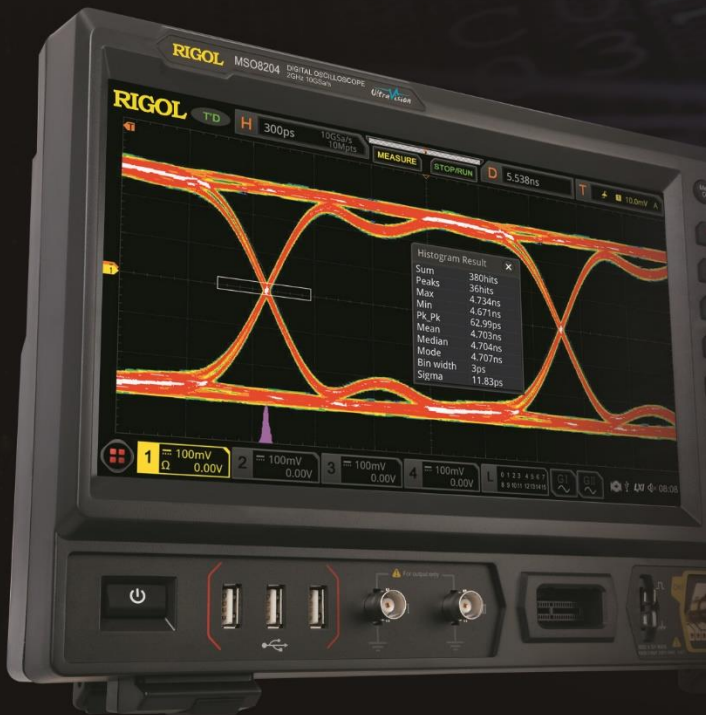
Perform eye measurement on the 622 Mb/s signal.
